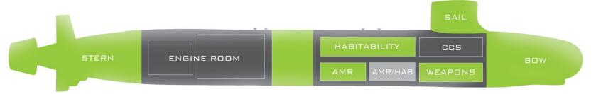
Newport News Shipbuilding builds the stern, habitability and machinery spaces, torpedo room sail and bow. Electric Boat builds the pressure hull, engine room and control room. Both build the reactor plant and alternate on the final assembly.
